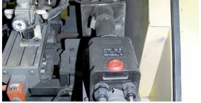
Deflashing foil sleeves from charcoal filter elements
